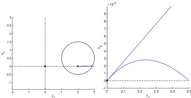
Fig. 5. Trajectory in a weak drift case with  $\mu = 0.5\|x_0\|$ ,  $x_0 = (2, 0)$  and  $x_f = (2.5, 0)$ . The final time is  $T \approx 0.56$ . Compare to Fig. 3. A zoom is given on the right-subgraph.
