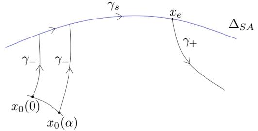
3) *Computation of the prior-saturation lift:* Actually, in the previous example, we can compute the prior-saturation lift with a smaller set of equations. The prior-saturation lift is the switching between the singular and positive bang arcs. What happens before is useless and we also do not need the matching equations. With these considerations we can set
