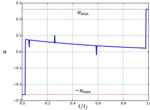
Figure 1: Control law for a time-optimal trajectory using direct methods obtained with a gauss discretization scheme of order 4 using 750 nodes. The control seems to follow a structure of the form  $\sigma_- \sigma_s \sigma_+$ .
