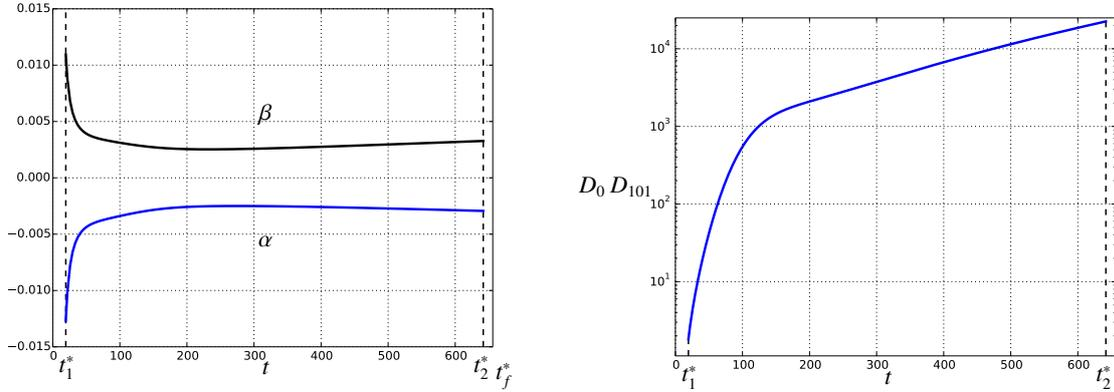
Figure 4: Evolution of the quantities  $\alpha(\cdot)$ ,  $\beta(\cdot)$  and  $D_0(x(\cdot)) D_{101}(x(\cdot))$  along the singular arc. The generalized Legendre-Clebsch condition from corollary 3.4 is satisfied all along the singular arc as  $D_0(x(\cdot)) D_{101}(x(\cdot)) > 0$ . The signs of  $\alpha(\cdot)$  and  $\beta(\cdot)$  along the singular arc confirm that we have an hyperbolic trajectory.
