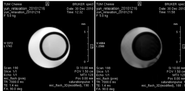
Fig. 1. Experimental results: The inner circle shape sample mimics the deoxygenated blood, where T_1 = 1.3s and T_2 = 50ms ; the outside moon shape sample corresponds to the oxygenated blood, where T_1 = 1.3s and T_2 = 200ms .
